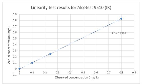
Figure 4. Linearity test for Alcotest 9510 (IR)
