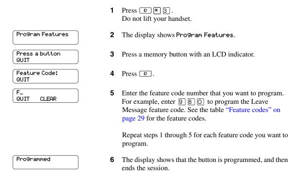
Use the paper labels that come with your telephone to identify the programmed button. To use the feature, press the labeled button.
