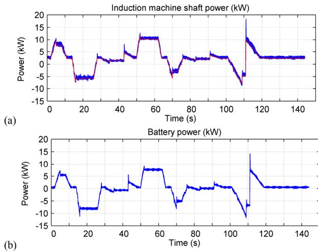
Figure 13. Measured waveforms of straddle carrier laboratory drive. (a) Induction motor shaft power, (b) battery power, (c) battery current, (d) battery SOC, and (e) battery current spectrum.
