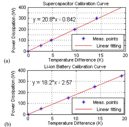
Figure 5. (a) Supercapacitor and (b) li-ion battery calibration curve.
