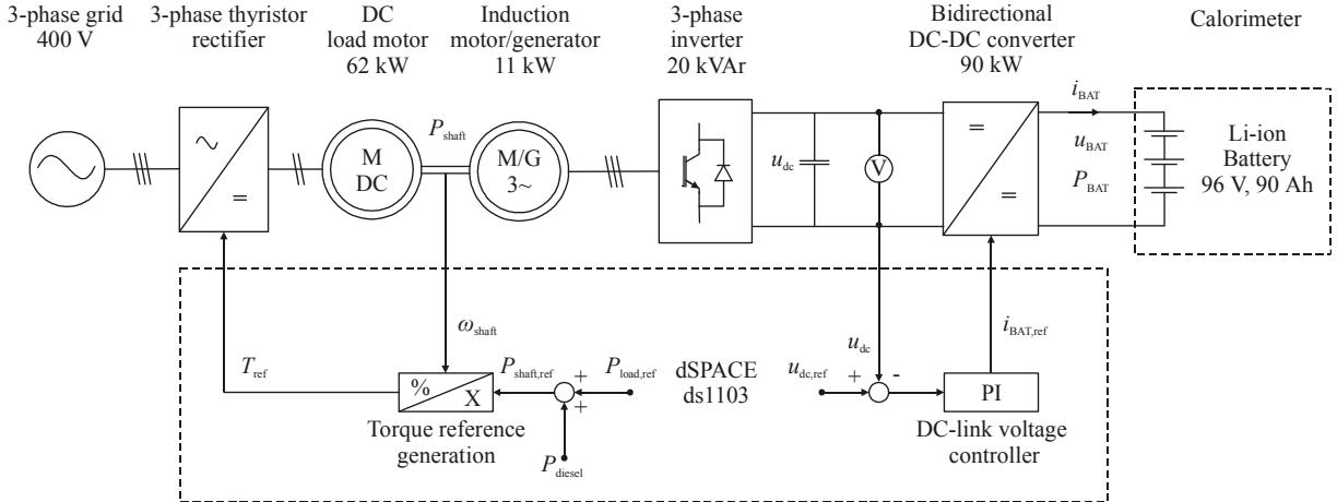
Figure 12. Laboratory drive for li-ion battery efficiency measurements with straddle carrier load pattern.
