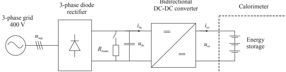
Figure 6. Test setup for energy storage efficiency measurements.
