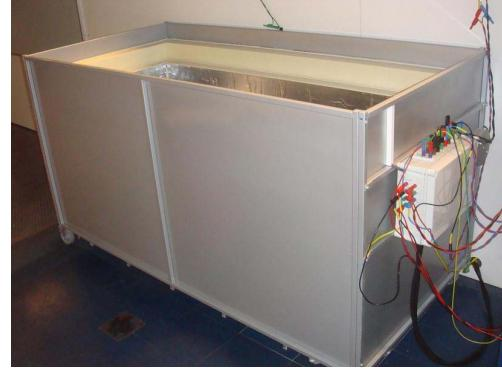
Figure 4. Balance calorimeter laboratory prototype.
