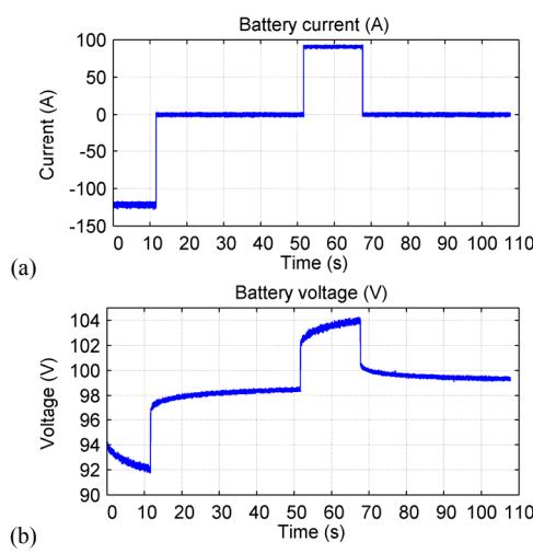
Figure 11. Battery (a) current and (b) voltage for determination of energy efficiency.
