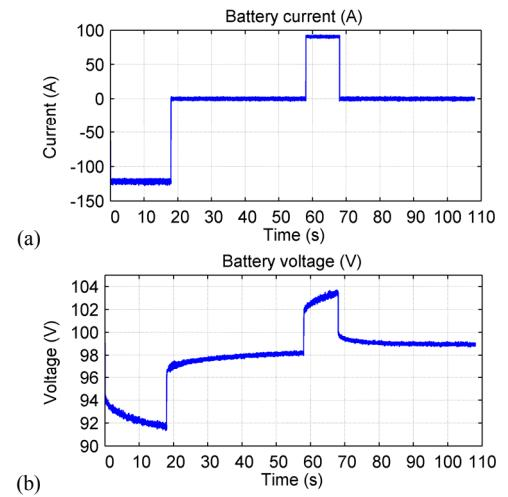
Figure 10. Battery (a) current and (b) voltage for determination of ESR.
