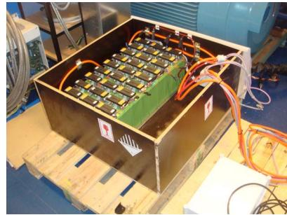
Figure 2. K2 96 V/ 90 Ah li-ion battery system of 30 pcs of LFP300HES Energy Modules.
