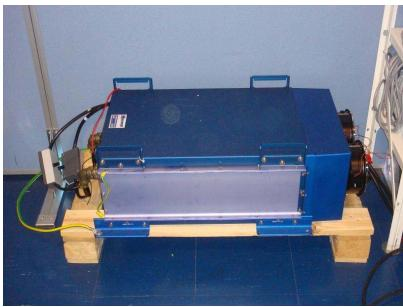
Figure 1. Maxwell BMOD0063 P125 V/63 F heavy-duty supercapacitor module.
