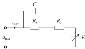
Figure 9. Dynamic li-ion battery model [14].
