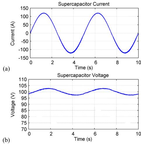
Figure 7. Supercapacitor (a) current and (b) voltage within test point  $I_{\text{es,rms}} = 84 \text{ A}$  and  $f = 0.2 \text{ Hz}$
