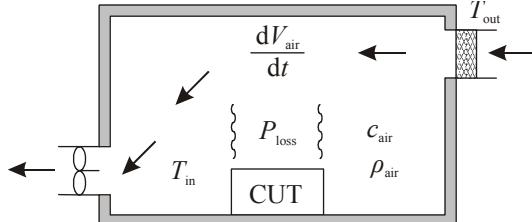
Figure 3. Balance calorimeter operation principle.
