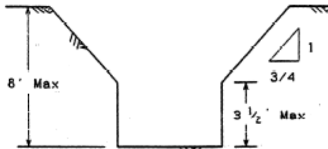
Unsupported Vertically Sided Lower Portion
