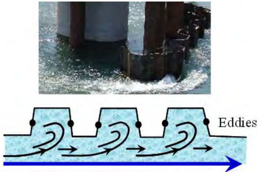
Figure 9-16. Hydraulic forces on cofferdams
