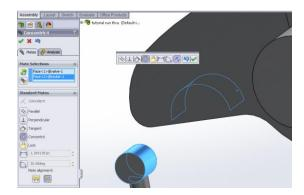
Now make a parallel mate with the right planes of the valve and the top bushing.
