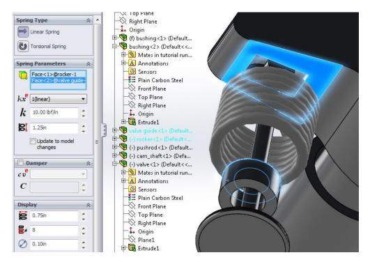
Click Okay and hit the recalculate button, you'll see the assembly's movement takes into account the motor and the spring.
