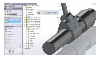
Now as you can see the pushrod and camshaft overlap, we need to use a mechanical mate and select the cam option.
