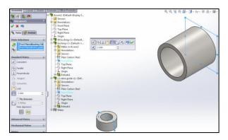
Insert the rocker and make a concentric and coincident mate with the top bushing (See below).
