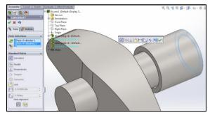
Insert the pushrod component and make a tangent mate between the rocker and pushrod. THIS STEP IS VITAL, DO
