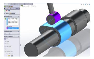
The next mate requires we bring in the valve component, mate it concentrically with the rocker as seen below.
