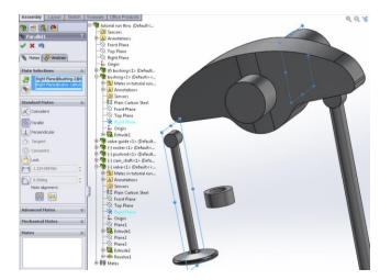
Make a 2 in Distance mate with front plane of the top bushing and the valve.
