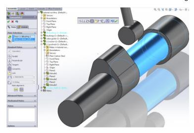
Coincident mate the front plane of the pushrod with the front plane o he camshaft
