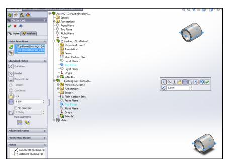
Bring a new component, the valve guide. Distance mate it to the top bushing with their right planes for 1.25 inches.
