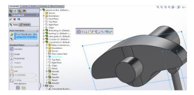
Insert camshaft and mate it coincident to the bottom bushing
