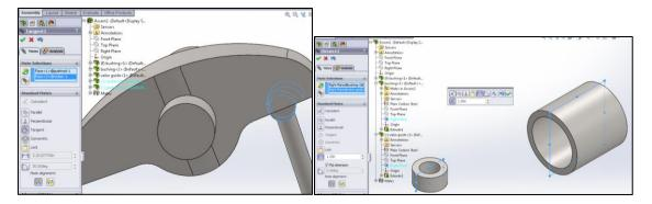
Make a distance mate of 1.25in between the right planes of pushrod and top bushing.
