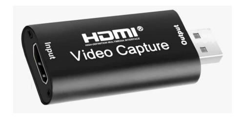
Connect the video capture card to your computer's USB port, and then connect the it with the analog DVR/camera via HDMI. If the DVR/camera does not support HDMI, e.g. if it supports S-video or VGA, then you can order a video capture card that supports S-video/VGA, or an S-video/VGA-to-HDMI converter.
