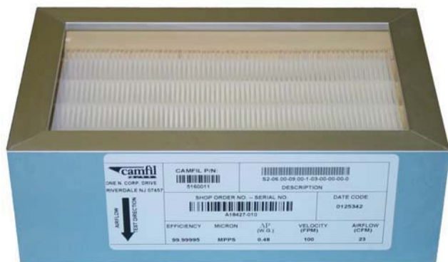
HEPA filter with label of test results.
