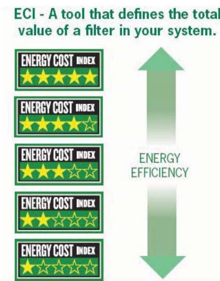
The above chart provides a relative comparison of the cost of energy to move air through the levels of star rated filters. Using a 5-Star final filter as opposed to a 1-Star final filter can save a facility up to $171.00 per year at 10¢ a kWh. Your system will vary based upon local kWh cost and system airflow.
