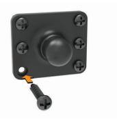
5 Press the socket in the device mount onto the ball of the wall mount until it snaps into place.
