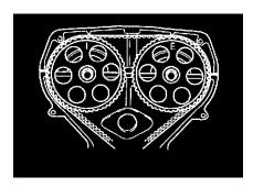
10. Check that "I" mark on intake camshaft pulley is aligned with mark on seal plate and "E" mark on exhaust camshaft pulley is aligned with mark on seal plate.
