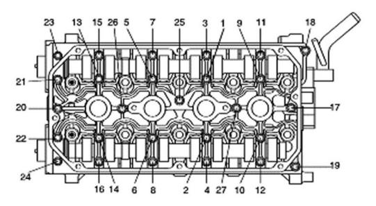
5. Install the cam carrier assembly. Tighten the cam carrier bolts as shown illustration. Tightening torque: 8.3 - 10.5 ft. lbs. (11.3 - 14.2 Nm, 1.15 - 1.45 kgf-cm)
