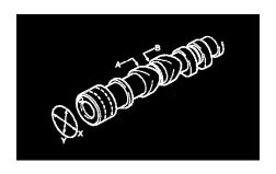
6. Check camshaft bearing journal diameter (X and Y directions) on both sides (A and B) of journal as shown in figure.
