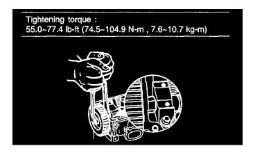
8. Install the camshaft pulley.
