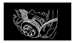
3. Check that timing mark on timing belt pulley is aligned with timing mark on engine.
