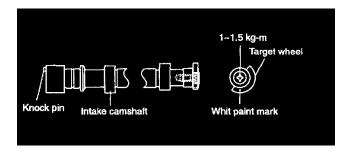
2. Install the phase sensor target wheel to the intake camshaft.
