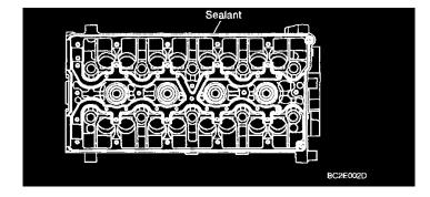
4. Apply liquid sealant on the cam carrier as shown illustration.
