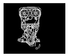
4. Check that "I" mark on intake camshaft pulley is aligned with mark on seal plate and "E" mark on exhaust camshaft pulley is aligned with mark on seal plate.
