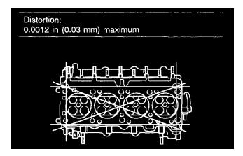
2. Measure cylinder head mating surface in six directions as shown in figure.
