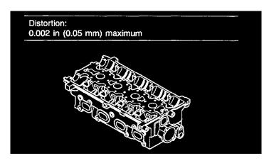
7. If distortion exceeds specification, resurface or replace cylinder head.
