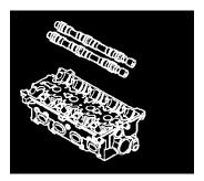
3. Install the camshaft after lubricating the journal of camshaft with engine oil.
