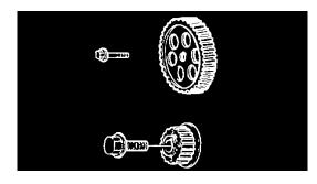
5. Inspect camshaft pulleys and timing belt pulley for broken teeth or damage.
