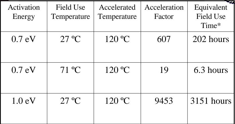
• Model is sensitive to difference in temperatures, activation energies.
