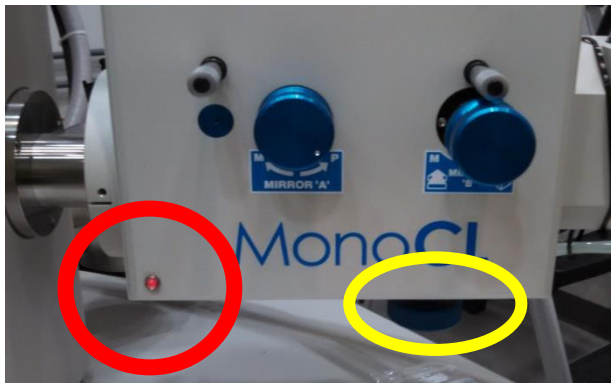
Red light.... The mirror is partially or fully extended. Mirror position knob is circled in yellow.
