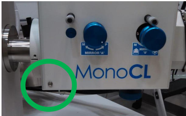
Green Light ....The mirror is fully retracted
