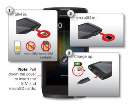
**Note:** To avoid SIM card damage, turn off your phone before you insert or remove the SIM card.
