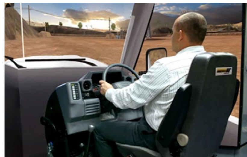
The physical exhibit can include elements from a real mining truck including a steering wheel, seat, shifter and levers for a realistic experience.
