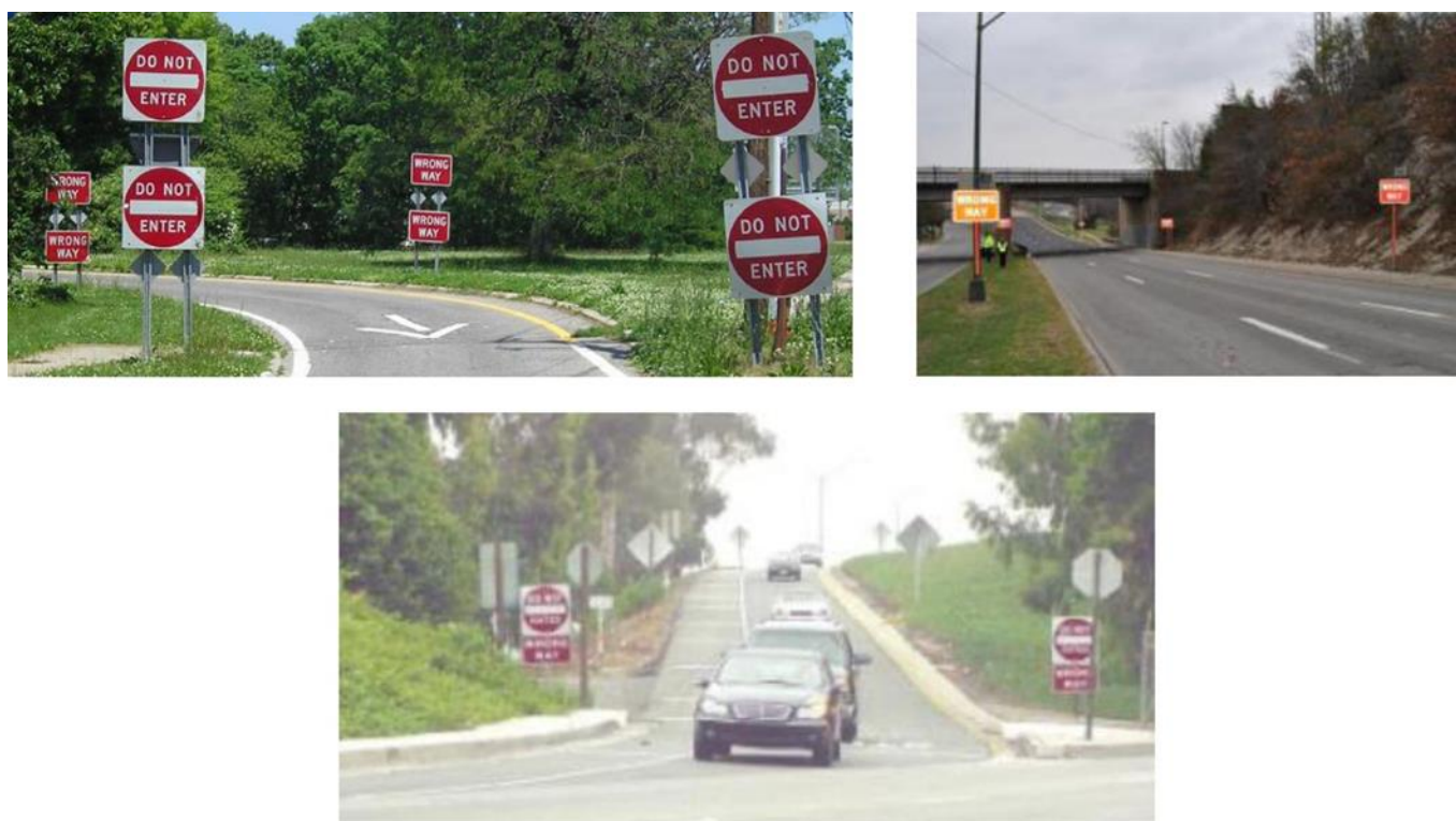
Figure 5.6.16–4: Examples of Wrong-Way Signage
