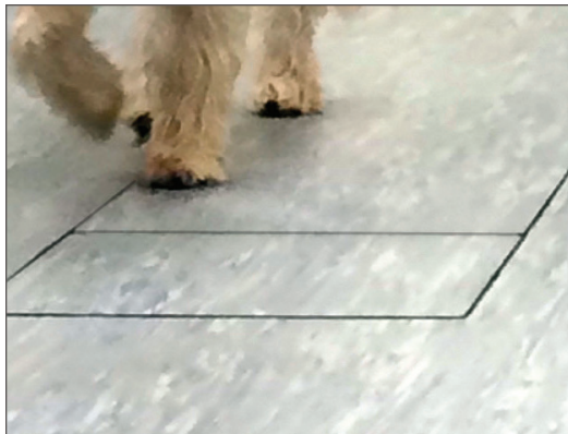
FIGURE 3. A force plate walkway; note the gray square in the center of the mat—this is the force plate that the dog must step on during the analysis.
