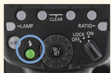
When the charging indicator is lit green, Quick flash is available. However, this is not available during Manual Flash.
