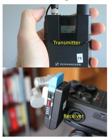
The Sennheiser AVX wireless clip-on microphone must be plugged into a transmitter.
