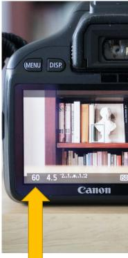
To adjust the shutter speed, move the dial on top of the camera.
