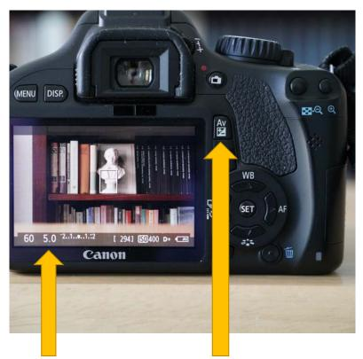
To adjust the lens aperture opening hold down the A/V button on the back of the camera and turn the dial on top.
