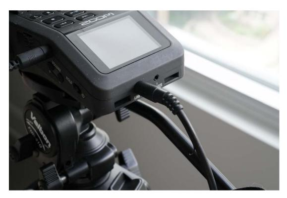
The Zoom recorder has an analog line output to send the audio signal to another device while it is simultaneously recording audio to the SD card.
