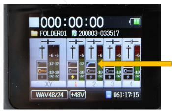
The microphone is plugged into input 2. The lo cut filter is indicated by a blue line.
