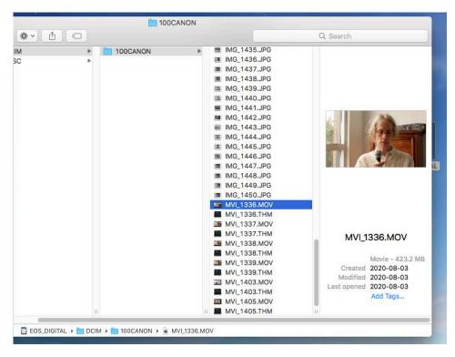
The camera records video using a H.264 codec (45-50 mbps) in the .mov container. These files will open up in QuickTime Player, VLC media player or any video editing program, including iMovie.
