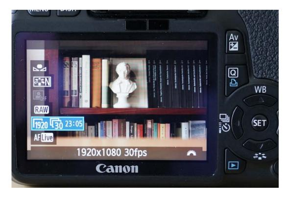
The Movie Recording Quick Menu Setting also displays the amount of recording time left on the SD card.
