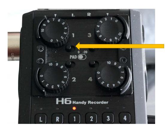
Adjust the volume for each microphone input on the front of the Zoom recorder.
