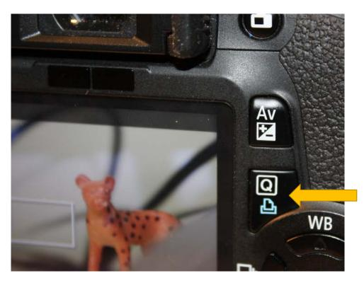
The Quick Menu displays common settings in the LCD display:
