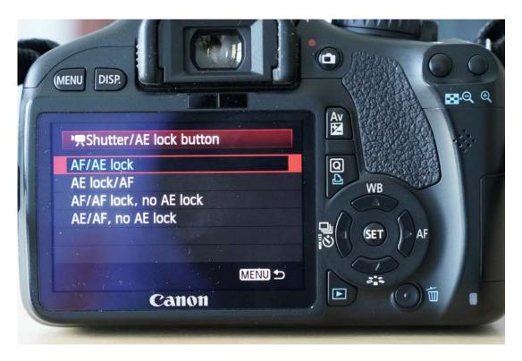
Set Shutter/AE lock Menu setting to the AF/AE lock position.
