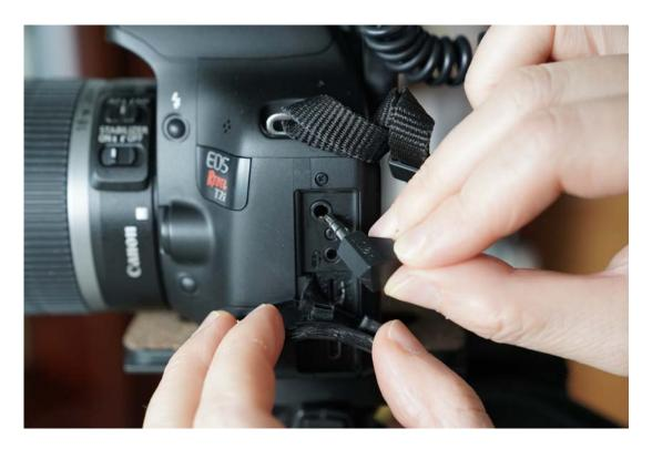
The microphone input is on the side of the camera.
