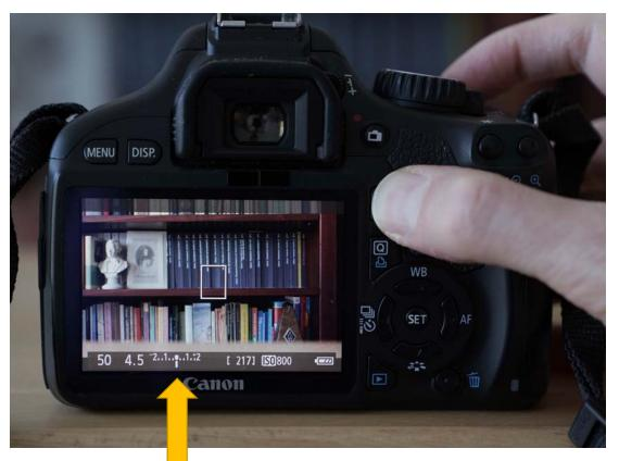
Holding the AV button on the back of The camera and turning the dial adjusts exposure compensation. When the dial lines up on the middle, the optimal exposure has been reached.
