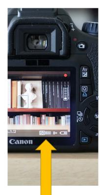
To adjust ISO, hold down the ISO button and turn the dial on top of the camera.
