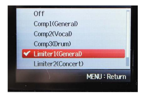
The MKH 416 is a very sensitive condenser microphone. I recommend putting a limiter effect on the input channel.
