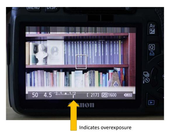
Here is an initial auto exposure performed by the camera. There are problems. First, the image is overexposed.
