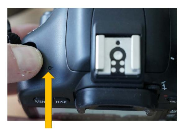
When focusing manually, you are calculating the distance from the subject to the camera's sensor, not the front of the lens.
