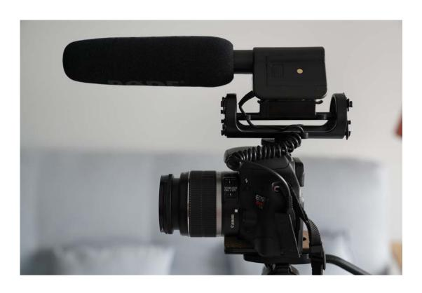
The Rode microphone is small mono directional microphone that can be mounted directly on the camera.
