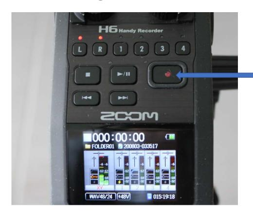
Adjust the recording volume level so that the audio peaks around -12 dB or between -12 and -6 dB.
