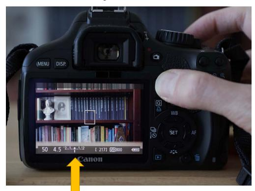
When the dial lines up on the middle, the optimal exposure has been reached.
