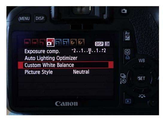
You may run into difficulties in a "mixed" lighting scenario, for example where there is a mixture of daylight and fluorescent or tungsten light. If none of the presets work, then perform a manual "custom" white balance.
