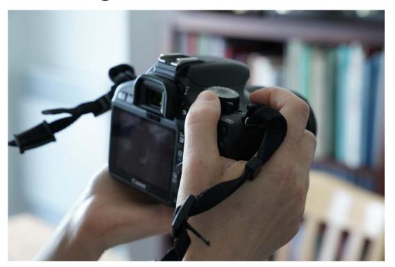
To minimize camera shake, turn stabilization on when you are hand holding the camera.
