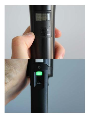
This is like a wireless SM58 microphone, but it has an omnidirectional polar pattern. It will pick up a little more room noise than the SM58. Position the microphone in the same manner as the SM 58 microphone.
