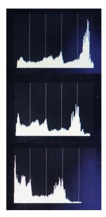
The histogram is used for judging the overall contrast of the image. Values increase in luminosity from left to right: shadows on the left, highlights on the right.
