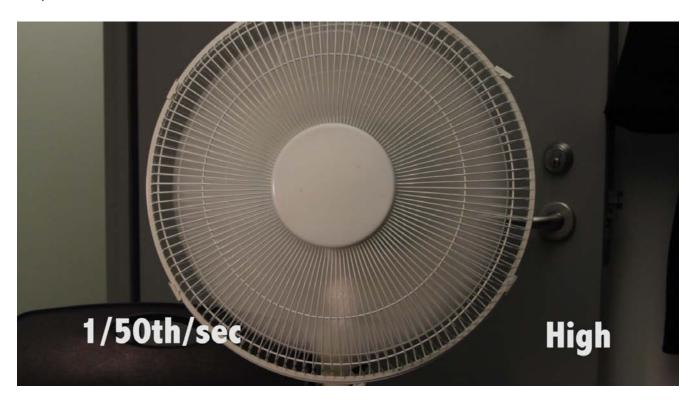
The fan is on high speed. The camera shutter speed is very high for 1080 24p video. The fan blades appear distorted. Normally all three are the same shape and size.
