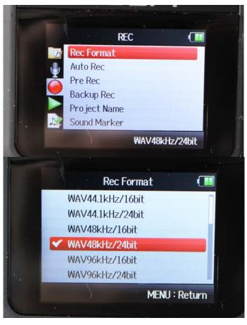
Record in the uncompressed WAV format. Do not use the MP3 format.
