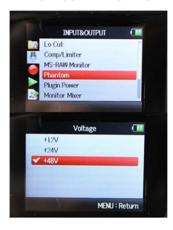
All audio devices that accept an input will have a "+48 V" button. This can be turned on to deliver "phantom power" to a condenser microphone. It should never be turned on when a dynamic microphone, like the SM58, is plugged into the channel.
