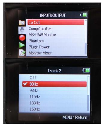
A low frequency cut filter can be added on an input channel in the Zoom recorder. Go into the INPUT/OUTPUT menu to add this effect. This will reduce the "proximity effect".
