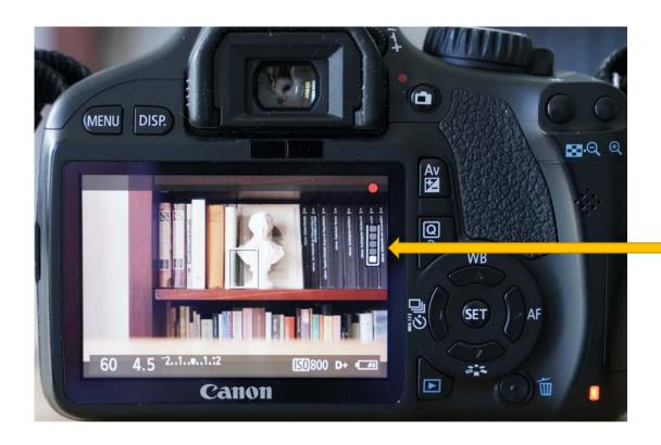
You'll notice that when you are recording there is a buffer (memory) indicator on the LCD. If the card is too slow to record video, the recording will stop and the indicator will have reached the top.
