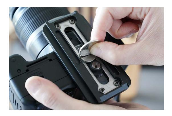
It helps to have a quarter handy to mount the tripod shoe on the bottom of the camera.
