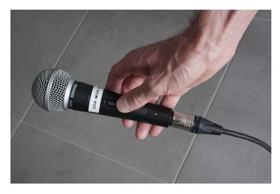
The Shure SM58 is a dynamic microphone. It does not require power to operate.
