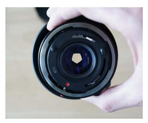
There is a metal leafed opening in the lens that lets in more or less light to the sensor (or to the film in an old film camera). This is the aperture. The smaller the number, the larger the opening.
