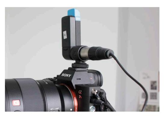
The XVX kit comes with a XLR to 1/8" adapter to plug the receiver straight into the input of a camera.
