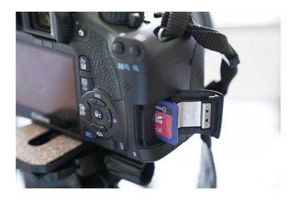
This model comes with a Class 10 8 GB SD card. This will record 22 minutes of HD video. Video can be recorded with a Class 6 SD card or higher.
