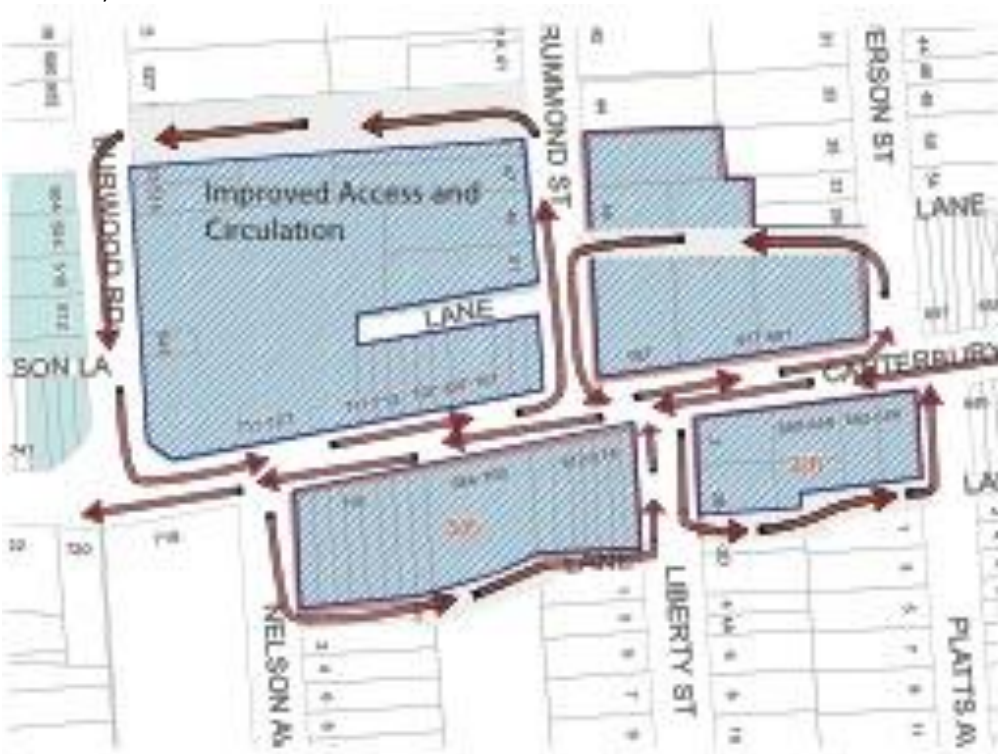
Figures 2e: How a typical road structure might be improved over time with left turn circulation (refer to Figure 2d above)
