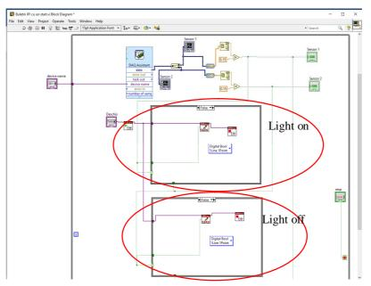
Fig. 8 – The diagram used to turn off the light.
