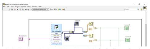
Fig. 5 – The diagram for the acquisition of the analogic signal and its transformation into a digital signal.
