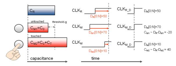
figure 3 Timing diagram of RC-delay line capacitance measurement method
