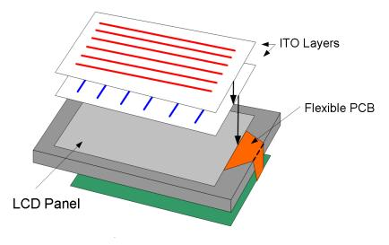
figure 7 Capacitive touch screen with matrix arrangement
