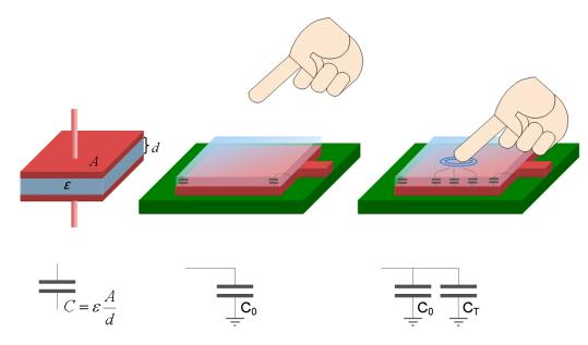
figure 1 Touch Sensor Principle: untouched sensor pad with parasitic capacitance  $C_0$ , touched sensor pad with additional touch capacitance  $C_T$ .
