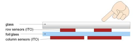
figure 9 High resolution capacitive touch screen with matrix arrangement, consisting of two ITO layers
