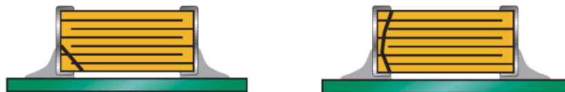
Fig.23. Angled crack between bottom of device to top of solder joint and fracture from top of device to bottom of device. source: AVX
