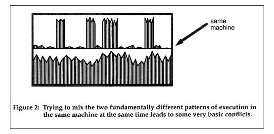
The patterns are simply incompatible. Either you get good response time and a low rate of machine utilization (at which point the financial manager is unhappy), or you get high machine utilization and poor response time (at which point the user is unhappy.)
