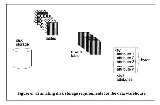
To calculate disk storage, first the tables that will be in the current detailed level of the data warehouse are identified. Admittedly, when looking at the data warehouse from the standpoint of planning, where little or no detailed design has been done, it is difficult to divine what the tables will be. In truth, only the very largest tables need be identified. Usually there are a finite number of those tables in even the most complex of environments.
