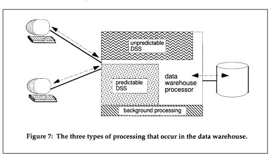
Background processing is that processing that is done on a predictable, (usually) batch basis. Typical of background processing is extract processing, data warehouse loads, monitors, sorts/merges, restructuring, index creations, etc. Background processing is that utilitarian processing necessary to the data warehouse but not directly associated with a query or an analysis of data warehouse data.
