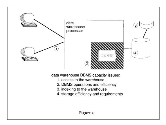
The capacity planner is interested in the access to the data warehouse, the dbms capabilities and efficiencies, the indexing of the data warehouse, and the efficiency and operations of storage. Each of these aspects plays a large role in the throughput and operations of the data warehouse.
