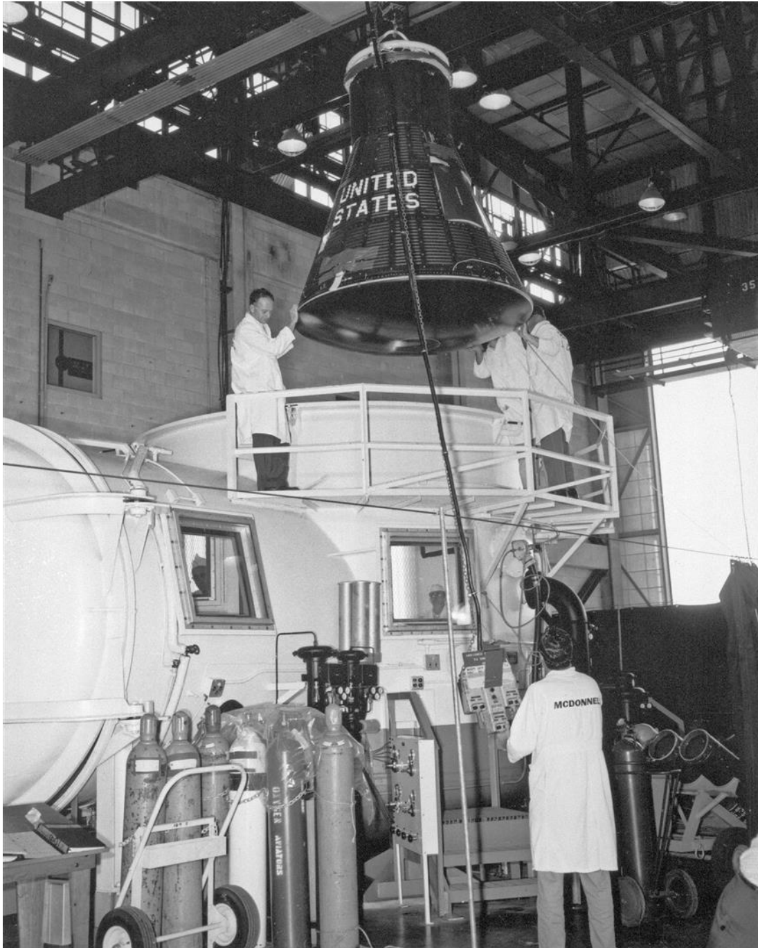
Figure 7. Mercury Capsule #16 being moved into the altitude chamber in Hangar S, 1962. (Courtesy of Kennedy Space Center Archives, Image LOC-62-3051).
