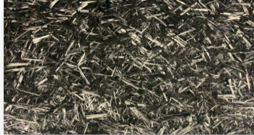
50k carbon fiber split to 3k
