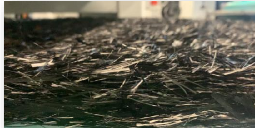
50k carbon fiber split to 3k
