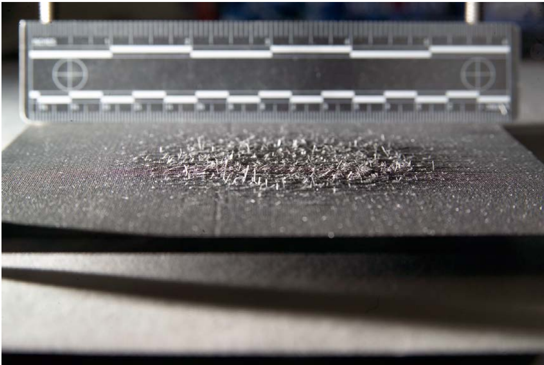
Figure 7 Small Scale Composite Surface after Hypervelocity Impact
