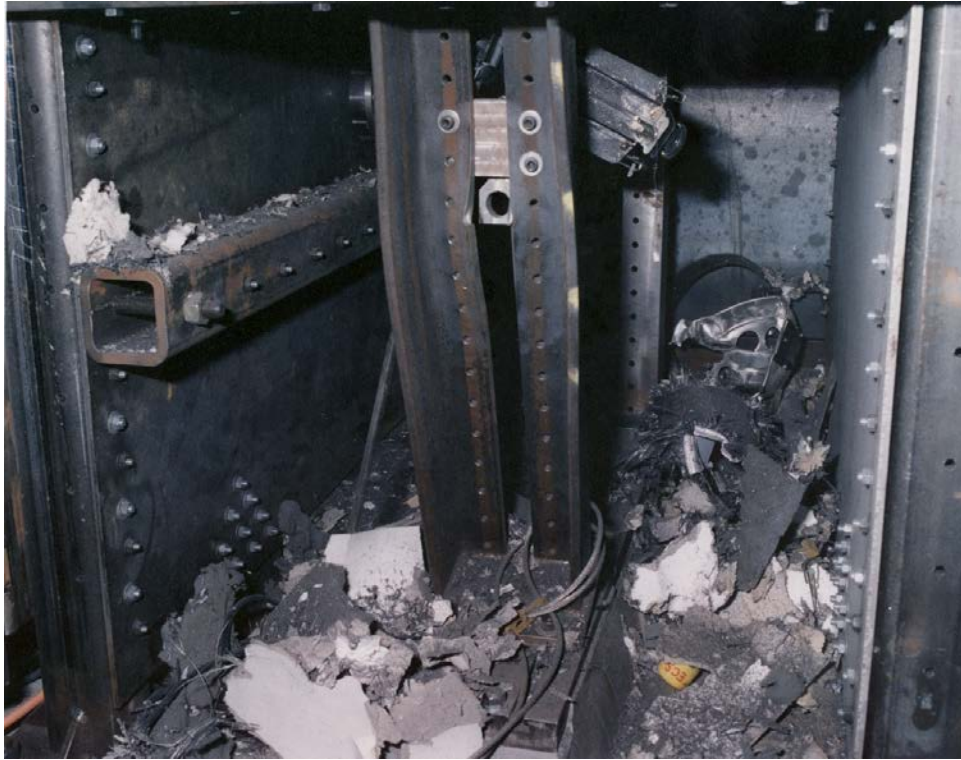
Figure 10 COPV Burst Dry Catastrophic Event
