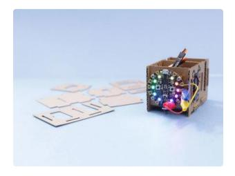
The enclosure is similar to cases that are designed to be made on a laser cutter. This design doesn't require screws or glue because of the tight tolerances in slots. Cardboard has a bit of flex so it can compress and fit through tight openings. The tabs extend beyond the slots to accommodate for slop during the cutting process.
