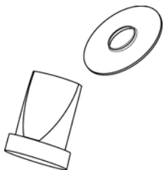
Figure 5.2 White Delrin retaining step washer and duck billed check valve
