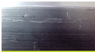
Die lines & surface damage
