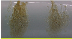
Pre-treatment water stain
