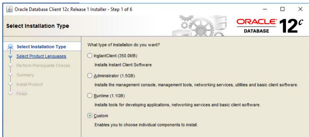
Figure 3-1. Universal Installer Installation screen. Select a custom installation. You may wait several minutes before reaching the next screen. Do not panic.
