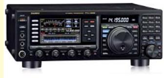
separation, the FT DX 3000 performance is 108.5 dB, IP3 +37 dBm. With frequency separation of only 2 kHz between the desired signal and an interfering signal, the dynamic range measures 106 dB and IP3 +33 dBm.
