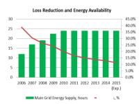
Energy Availability has increased to 24 hours on the Main grid. Technical and commercial losses have been reduced to 12% and should be further reduced down to 9% in pursuance with best engineering practice.
