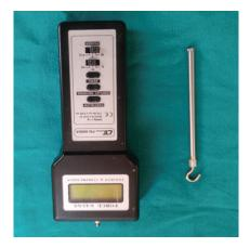
FIGURE 8: Digital force measurement gauge.
