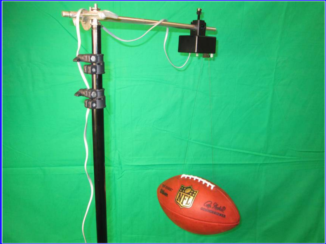
Figure 1.3: The hanger used to suspend the football is simply a lightweight string that has been woven under the stitches of the football. The string is then connected to a binder clip that is then suspended from the electromagnet.
