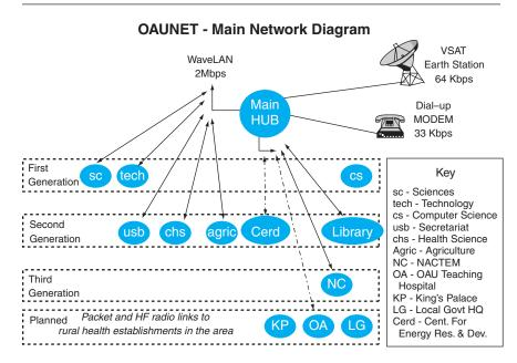
FIGURE 9-11 OAUNet in Nigeria: Main Network Diagram
