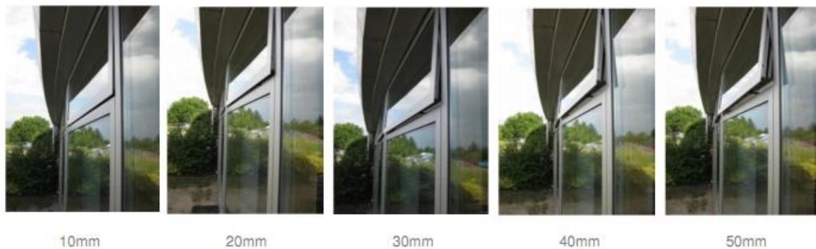
Figure 2. 4: Automated window opening with various opening width
