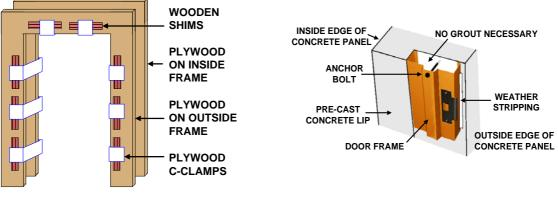
Figure 10: Diagram of Plywood Fix
