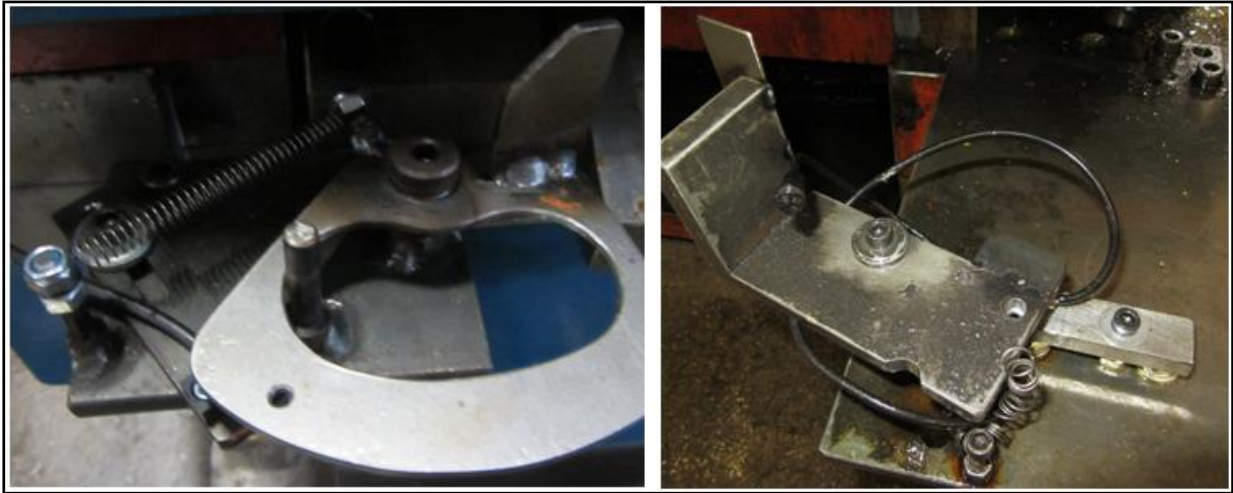
Figure 50: Sensors on the die
