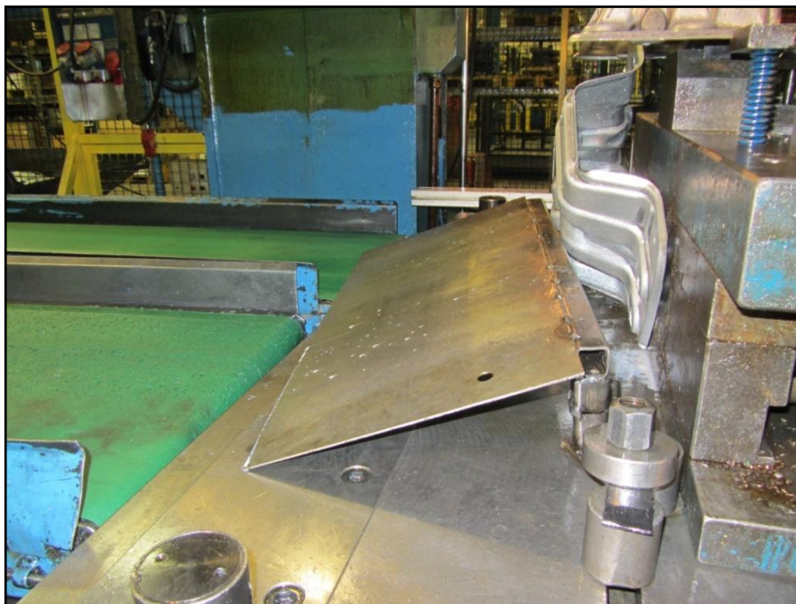
Figure 62: Ramp not fulfilling its task
