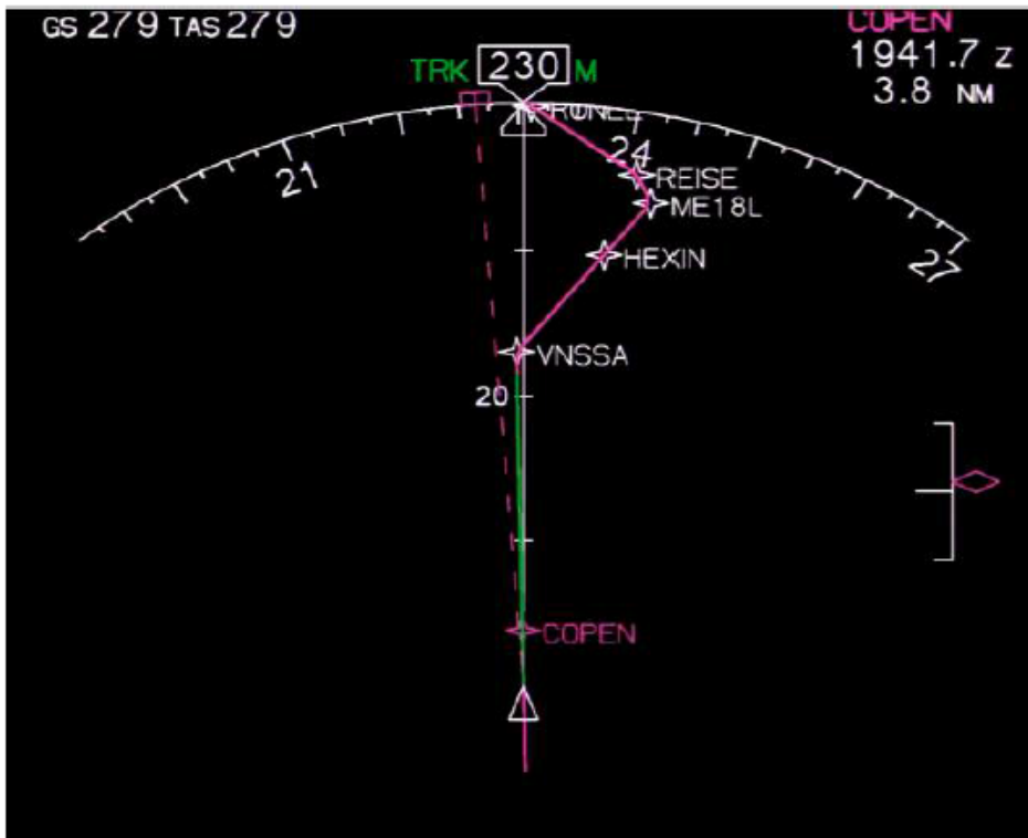
Trajectory prediction on the Navigation Display (ND) and Vertical Situation Display (VSD)
