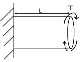
• To find the displacement of the cylinder, we use Castigliano's Theorem with the strain energy for torsion.
