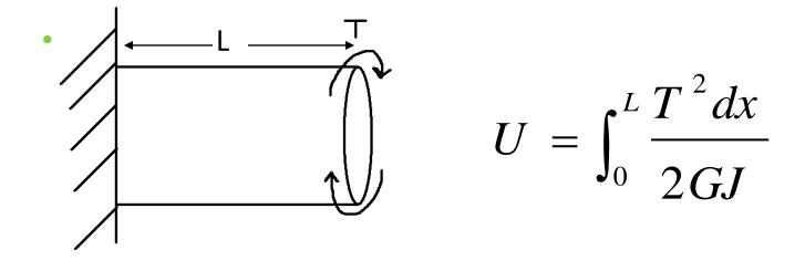
Where T is the torque applied, G is the Modulus of Rigidity, and J is the polar moment of inertia.
