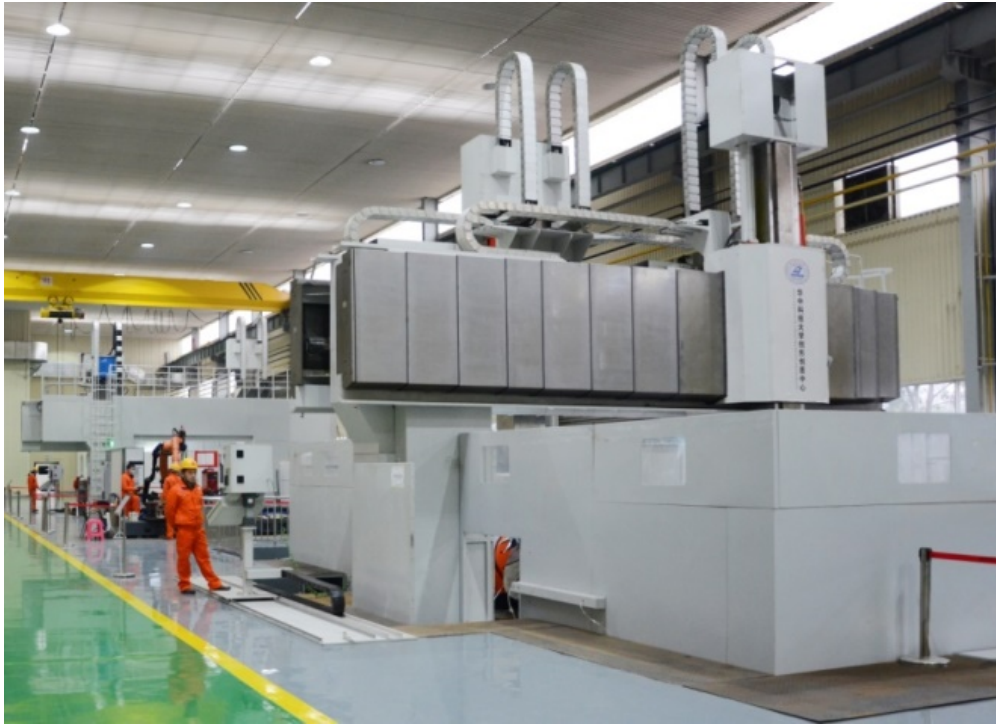
Fig. 3 Equipment for CFMC additive manufacturing
