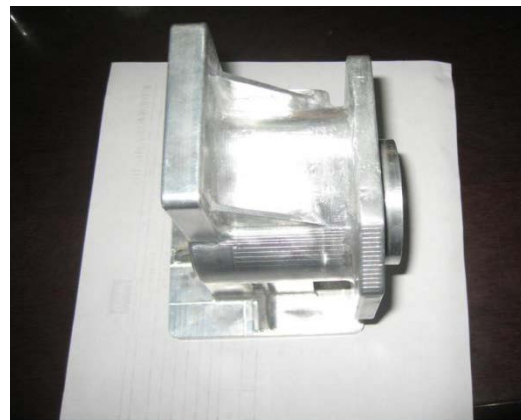
(b) An aeronautical part from high-silicon aluminum alloy
