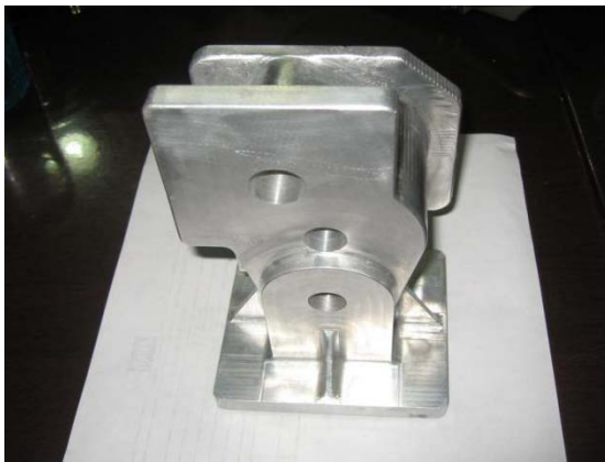
(b) An aeronautical part from high-silicon aluminum alloy
