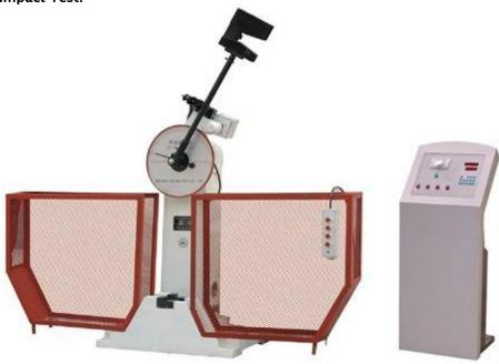
In this test the casting is subjected to a blow from a hammer of known weight striking or falling on the casting. Defective castings fail under the impact of the blow but the method is very crude and unreliable.
