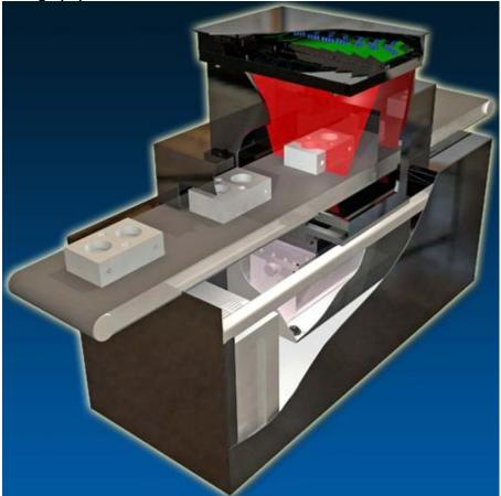
Radiography uses X-rays or gamma rays penetrating through the castings and giving a shadow picture on a photographic film placed behind the work piece. These rays have very short wave length of the order of 0.001 Angstrom ( $10^{-10}$ m) units to 40 Angstrom units for x-rays and 0.005 to about 3 Angstrom units for gamma rays compared to about 5500 Angstrom units for the centre of the visible spectrum.
