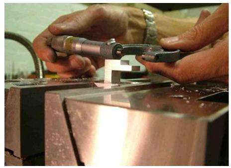
Dimensional inspection is carried out to make sure that the castings produced have the required overall dimensions including allowances for machining. It may sometimes be necessary to break a part of the casting to take measurements of inside dimensions.
