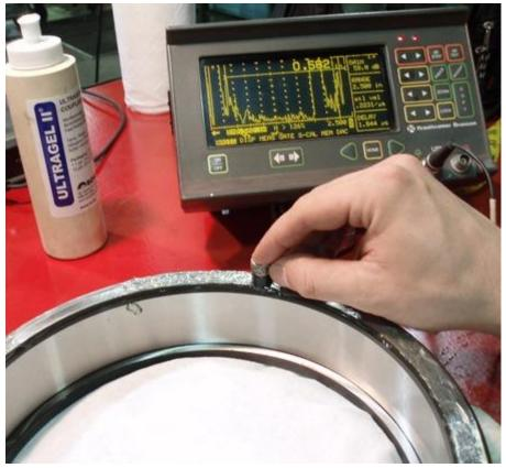
The time interval between the transmitted ray and reflected ray is recorded by a cathode ray oscilloscope. Any crack or void in the casting results in reflection or some of the sound from the crack which appears as a pip between the two pips representing the thickness of the casting. The depth of the crack from the surface of the casting can be easily calculated from the distance between these pips.
