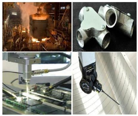
In process inspections are carried out before a lot of castings have been completed to detect any flaws that may have occurred in the process so that corrective measures can be taken to remove the defect in the remaining units. Finished product inspections are carried out after the castings have all been completed to make sure that the product meets the requirements specified by the customer.
