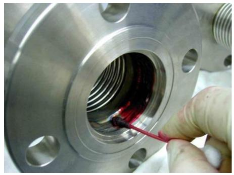
After the penetrant has been applied to the surface to be tested extra penetrant is wiped off the surface is dried and a developer applied to it. This developer helps in drawing out the penetrant so that it becomes visible on the surface. The penetrant liquids often contain materials which fluoresce under ultraviolet light or a die to indicate their presence.
