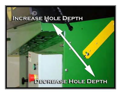
• Note: Moving the bar too far up or down will trigger a micro switch and keep the machine from cycling properly. If this happens adjust in the reverse direction slightly and try a test piece. This is a trial and error adjustment.
