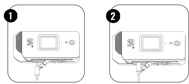
1. Open the USB port cover, connect the USB power cable to the charging power adapter and insert USB cable into USB port.
