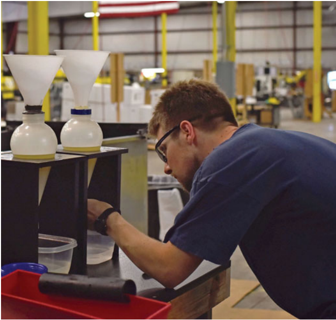
Schier engineer lab testing a grease interceptor
