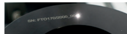
Figure 15: Engraving of black anodized aluminum
