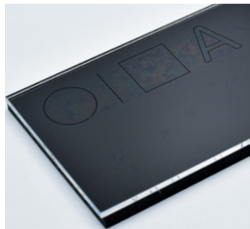
Figure 6: Microstructures in laser transmission welding
