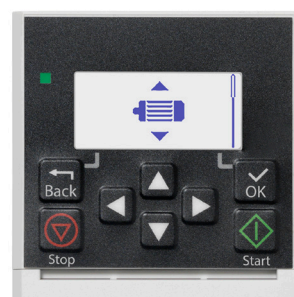
The built-in icon based control panel interface for easy commissioning and configuration
