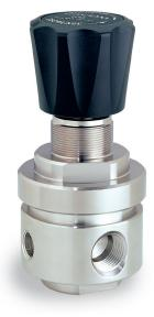
TESCOM 44-3200 Series is a compact, high flow, high purity single-stage regulator for specialty, flammable and industrial gas flows of 5-50 SCFM / 141-1415 SLPM. Diffusion-resistant metal diaphragm seal ensures gas purity and integrity.
