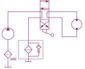
Figure 1(b). Return Line Filtration Circuit
