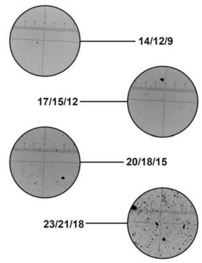
Figure 2. Microscopic Particulate Comparison
