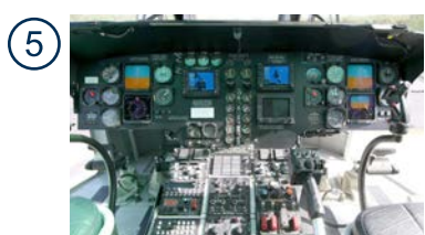
Rockwell Collins Four (4) Display FDS Electronic Flight Instrument System Upgrade with Dual AHRS
