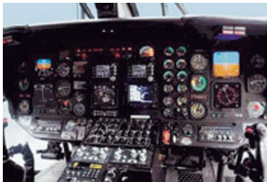
Rockwell Collins Four (4) Display FDS Electronic Flight Instrument System Upgrade with Dual AHRS
