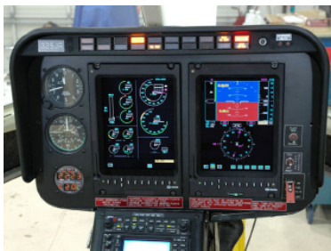
SAGEM Electronic Flight Instrument System and AHRS Upgrade
