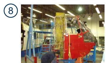
Fifty Inch Section Removal from Forward Fuselage between Stations 110 and 160
