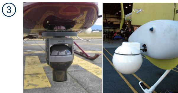
- Nose-Mounted Tokimec/Cineflex Gyro Stabilizer E.N.G Camera - Tokimec Antenna Array
