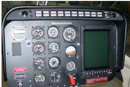
Single SAGEM Avionics ICDS-8 Integrated Cockpit Display System with Attitude and Heading Reference Inputs and a Garmin GNS430 NAV/COMM/GPS System
