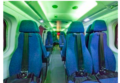
Helicopter Emergency Egress Lighting (HEEL) System
