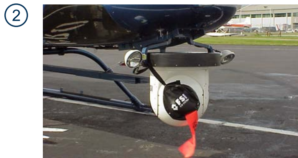
- FSI Ultra Media II or III, or Wescam 16SS-320, 16SS-B750/725, 16SS-1000, 16DB-750 Camera and Isolation Mount - FSI Ultra Media II Camera and Isolation Mount
