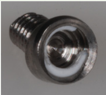
Extragate Titanium Abutment inclined at 15° without screw. The white Seeger must be positioned with its open side towards the Extragate bevel.
